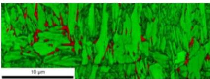
[Microstructure of a Q&P steel]
