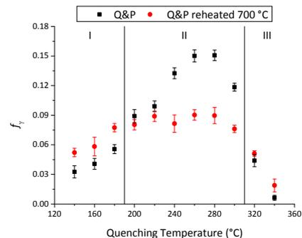
[Retained austenite in a Q&P steel before and after reheating to 700°C. MSc Thesis of T. Koopmans, 2015]
