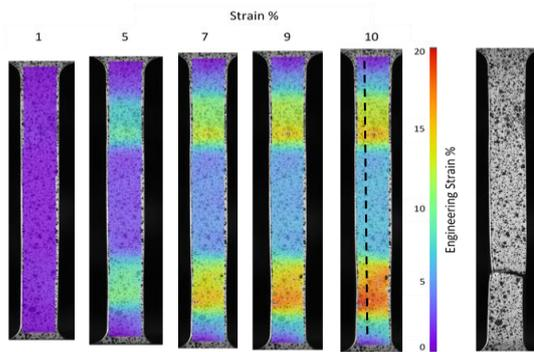
Figure 2. Digital image correlation showing evolution of local strain as a function of cross head displacement (shown for gradient depicted fine grained matrix and two coarse highly oriented grained regions)
