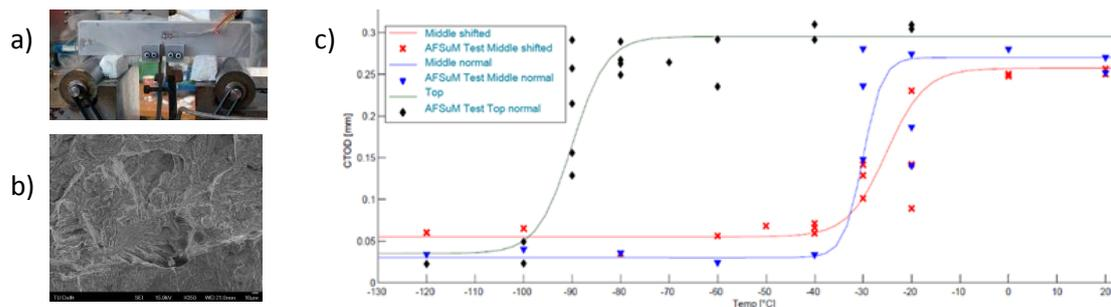
Figure 3. a) sub-sized CTOD test b) cleavage facets and the inclusion, as a crack initiation site c) fracture toughness (CTOD) results of the HAZ of welded plate (red curve refers to top, blue to middle)
