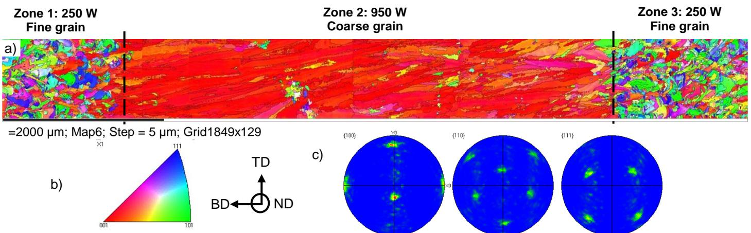
Figure 1. EBSD analysis of a graded Inconel 718 featuring single coarse columnar grain zone embedded in a fine grain matrix a) Inverse Pole Figure (IPF) coloured map of Y-Z section b) The index map of IPF and the reference coordinate c) Pole figures texture for zone 2.
