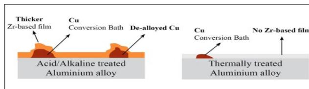
The surface chemistry of metal (oxides) highly influence the deposition mechanism and kinetics of Zr-based conversion coatings
