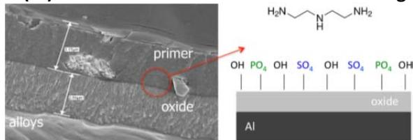
Cross-sectional and schematic view of the metal-oxide-primer interface
